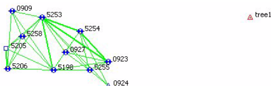
Figure B-8. Control Point (Tree1) Not Linked with Network
