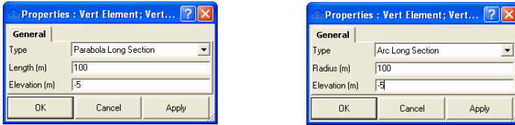
Figure 9-64. Add Vert.Element: Long Section Dialog Box. General Tab
