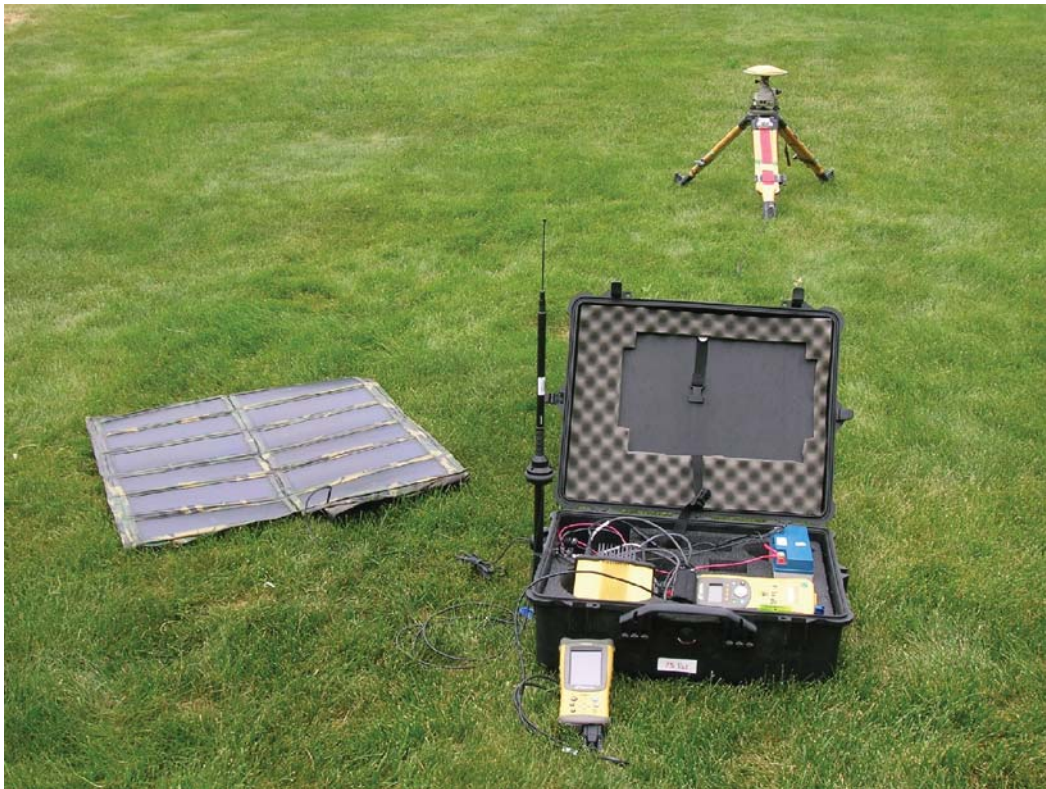
Battery and solar-powered RTK base station with Topcon GB-1000 Receiver, PG-A1 GPS Antenna, and FC-100 Data Controller. Radio antenna (left of case) has not yet been mounted.
